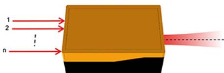
Figure 8 : Non-coherent combiner principle
