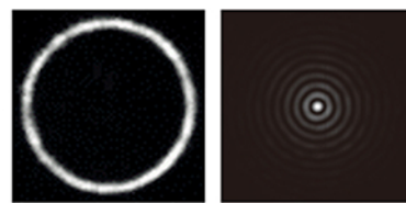
Figure 6 : Measured circle beam profile (left) and Bessel beam at far field (right)
